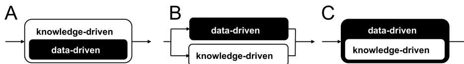
Figure 1: Typology of hybrid models (see von Stosch et al. [16]). A and C represent serial structures: under A, a data-driven model is used as input to a knowledge-driven model; C is the reverse. B represents a parallel structure in which knowledge-driven predictions are corrected by data-driven predictions.
