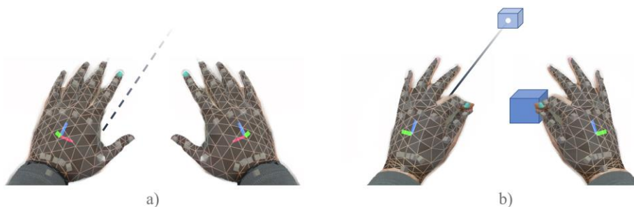
Figure 8 – The MR input system and hand gestures for near and remote interactions. a) Neutral position, Hover, and touch. b) Grab, move, and rotate.
