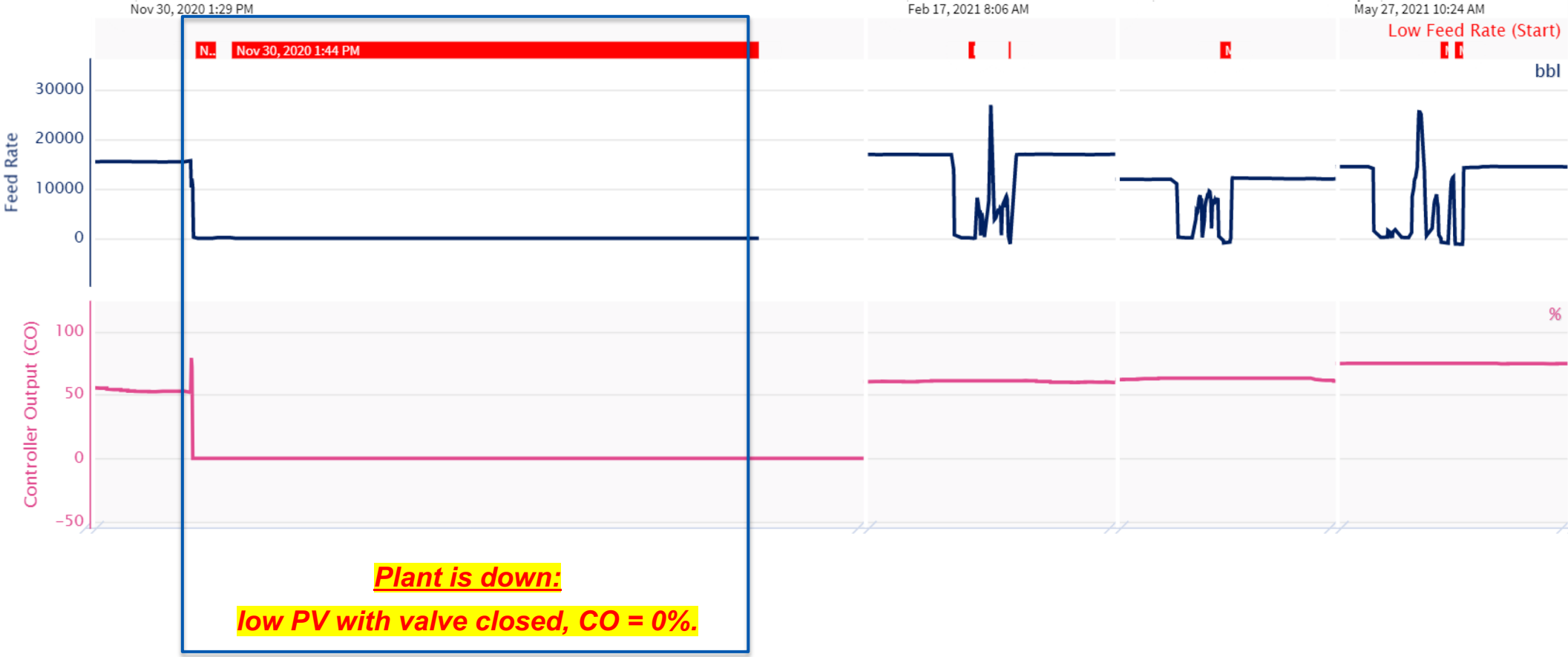
Figure 9: Time series of feed rate (PV, blue), feed rate controller valve output (CO, magenta), and regions with feed rate < 100 BPD (red)
