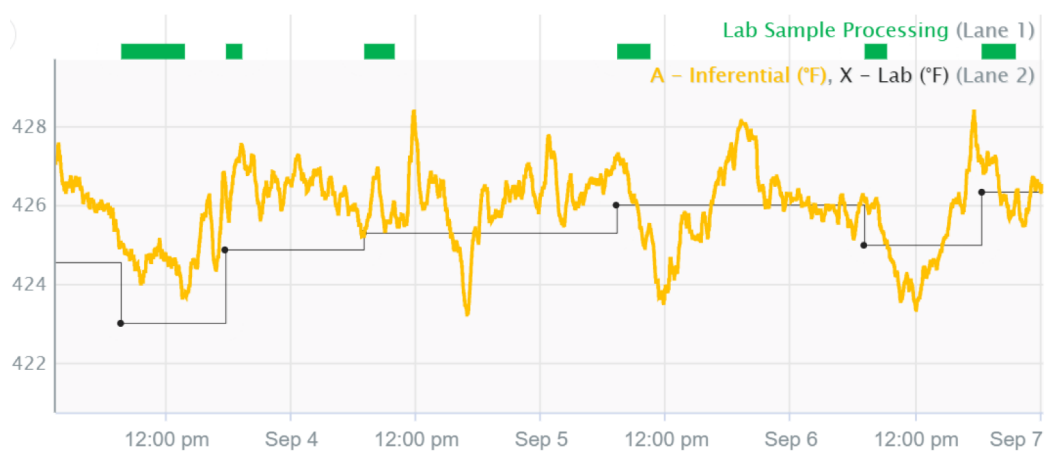
Figure 14: Time-series of inferential prediction (high frequency), lab results (twice daily) and time required for lab sample processing (green bar).
