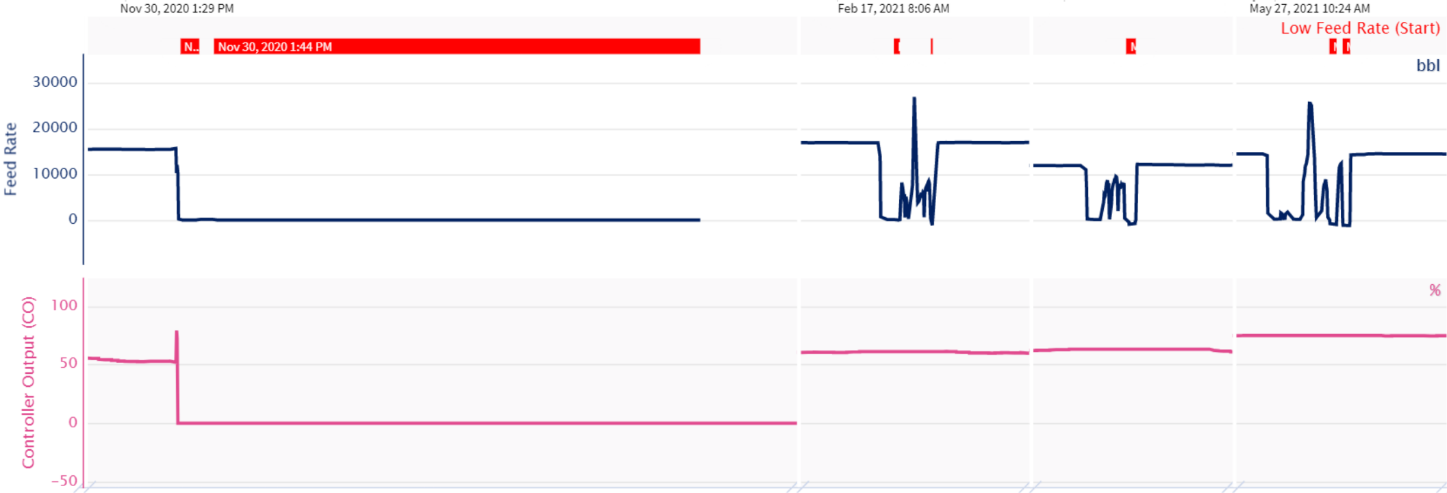
Figure 9: Time series of feed rate (PV, blue), feed rate controller valve output (CO, magenta), and regions with feed rate < 100 BPD (red)
