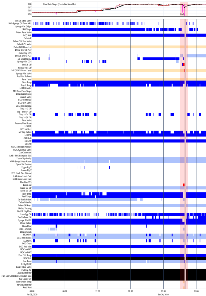
Figure 12: Combined DCM and time series trends for Case Study 1, investigating a process upset in the FCC feed rate. The time window under investigation is highlighted in light red. We can observe that the majority of variables did not experience any constraint changes. These variables are unlikely to be direct contributors to the feed rate drop, and can be removed to narrow down the list of variables for further investigation.
