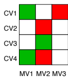
Figure 1.8: Sample system to illustrate the proposed generic controller diagnosis process. The steady-state gain matrix shows the directions of each MV/CV pairing, with negative gains in red and positive gains in green.
